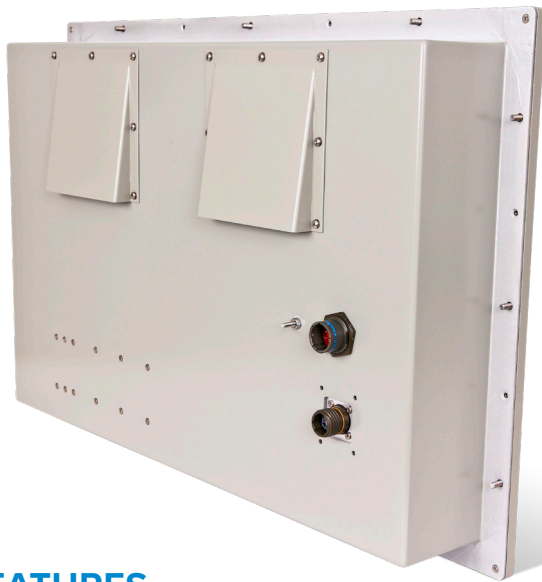
Mil-spec Saber PanelMount 24.0 includes a 1/2" thick front bezel, mil-grade connectors, and rear louvers to protect fans
