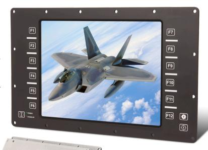
Mil-spec Saber PanelMount Solar 10.4 UPB shown with custom bezel buttons, and lacks a rear enclosure to simplify mounting
