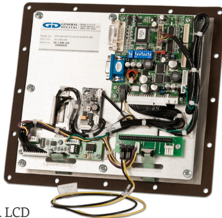
Mil-spec Saber PanelMount Solar 6.5 UPB shown with custom bezel buttons, and lacks a rear enclosure to simplify mounting
